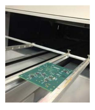
For an oven to achieve the required reflow profile suitable for a specific solder paste, it may be necessary to tweak its controls based on the PCB assembly being soldered. Major factors causing the variations are:
