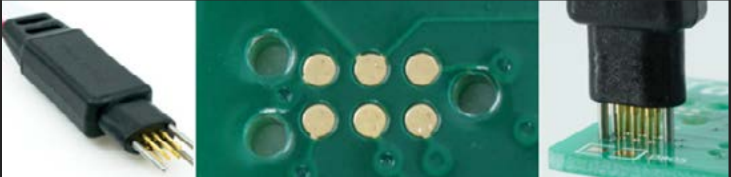
This set of images from tag-connect.com shows the head of the programming cable, the footprint, and the two devices connected.
